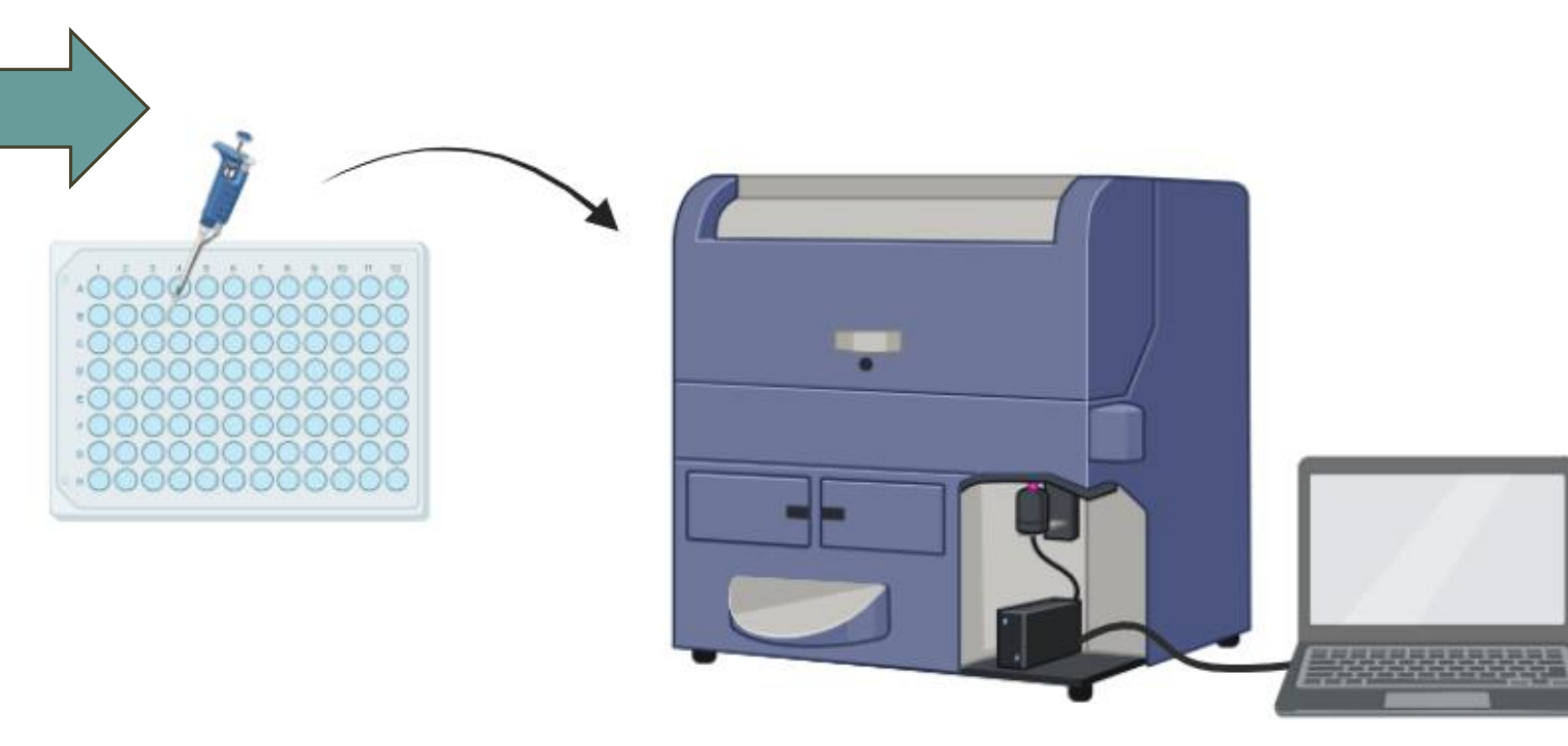
Figure 4. A flow cytometer run setup for measuring the spore and host abundance in cells/mL.
