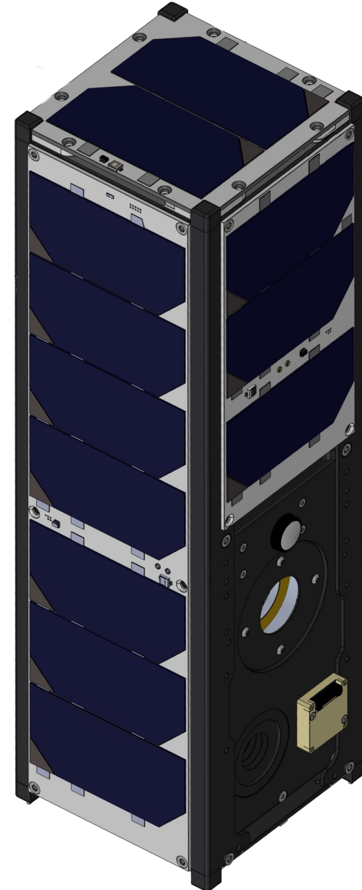
Figure 1: 3UCubed CubeSat CAD model
