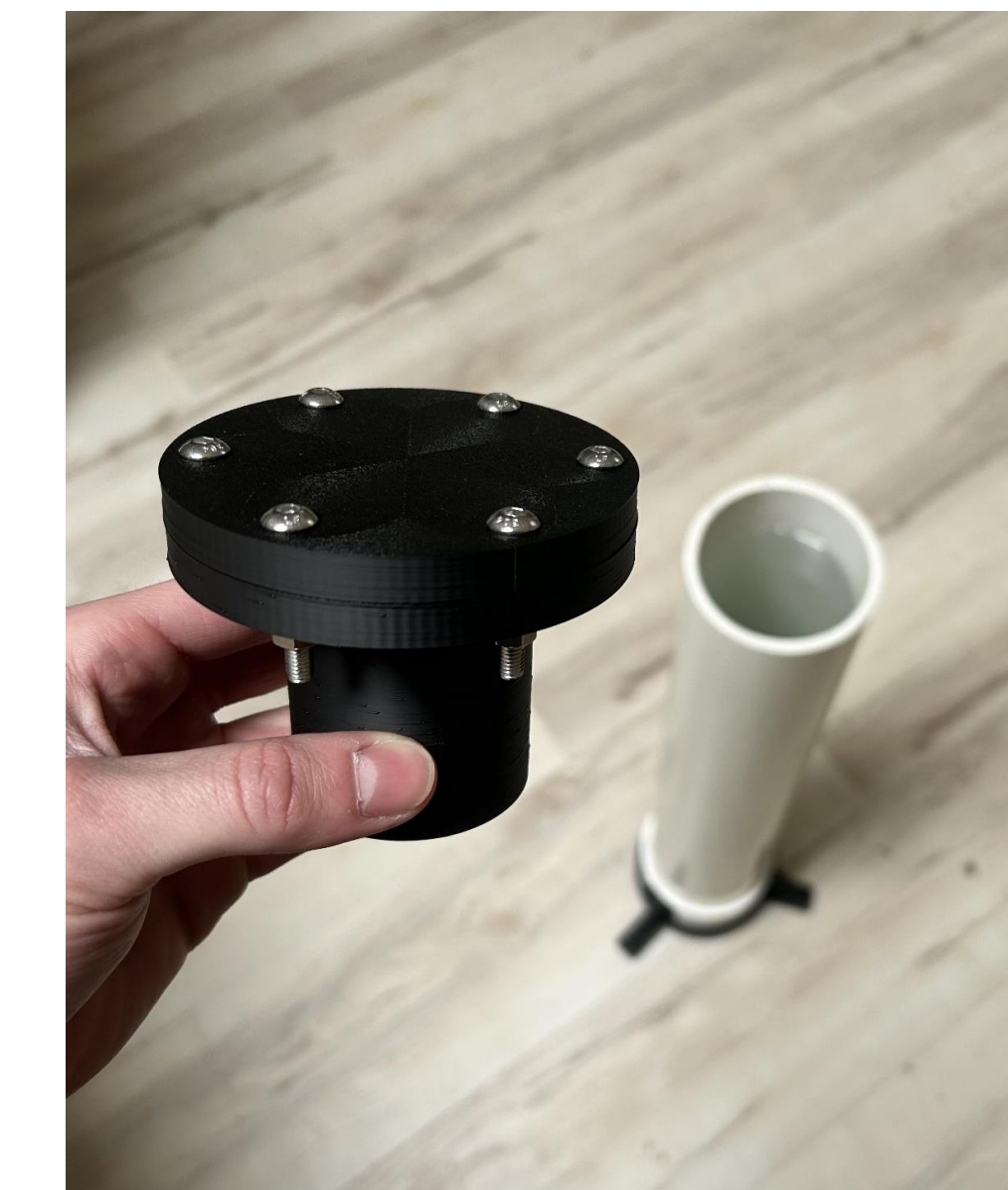
Figure [7]: IP67 Submersion Test. The 3D-printed antenna chamber held over a custom-built 1-meter water column to validate seal integrity and hydrostatic pressure resistance for 30 minutes.
