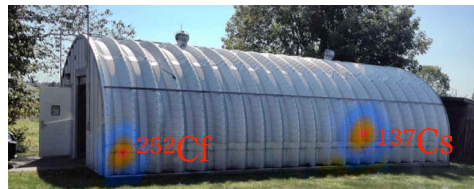
Simultaneous imaging of neutron (left) and gamma-ray (right) sources.
